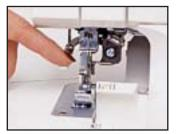
**Needle Threader:** Needle threading is quick and easy. A touch of a lever automatically threads the eye of each needle.
